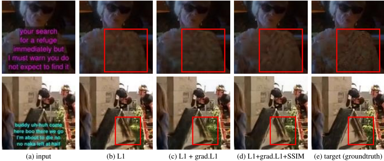
Figure 3. The impact of each loss terms. (a) An input center frame. (b-d) The reconstructed frames with: (b) L1 loss, (c) L1 + gradient L1 loss, and (d) L1 + gradient L1 + SSIM loss. (e) Ground truth frame. Best viewed when zoomed-in.
