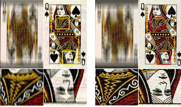
**Fig. 19** Comparison of the deblurring performance with different sequence lengths under the same exposure. (a) sequence length = 40, 1 chop duration = 3 ms. (b) sequence length = 120, 1 chop duration = 1 ms.
