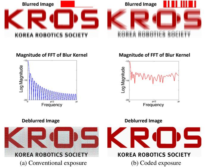
Fig. 2: Comparison between conventional exposure and coded exposure. (a) A poor deblurring result due to non-invertible blur kernel, (b) Coded exposure shows a good deblurring result.
