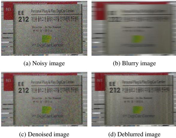
Fig. 1: An example of a motion blur in a mobile robot. Both images (a,b) are captured from a moving mobile robot under low light condition. (a) short exposure time and high ISO sensitivity settings are used to avoid motion blur and it amplify image noise. (b) Long exposure time is used to prevent image noise and it cause severe motion blur. (c) image denoising result of (a) using median filter, (d) image deblurring result of (a) using Wiener deconvolution (MATLAB).
