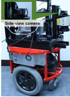
Fig. 5: Our mobile robot which is used for the experiments. The robot captures images sequentially using a side-view camera.
