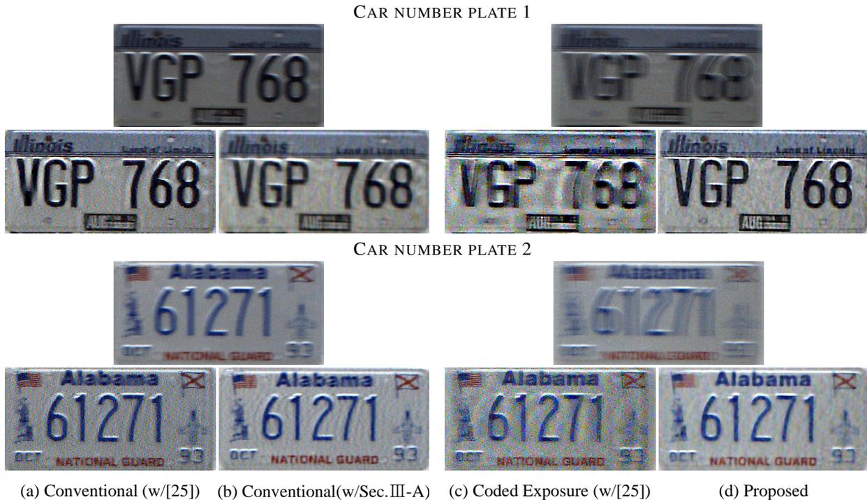
Fig. 6: Qualitative comparison of deblurring results. (a) Conventional exposure with [26] fails to recover details and to suppress deconvolution noise. (b) Conventional exposure with Sec. 3.1 results in ringing artifacts due to a loss of spatial frequencies of the blurred images. (c) The method [26] fails to estimate accurate blur kernels. (d) The proposed method shows promising deblurring results.
