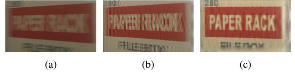
Fig. 4: Handling a simple projective blur. (a) Input image. (b) Deblurred result assuming spatially-invariant blur kernel. (c) Deblurred result using Sec. 3.2
