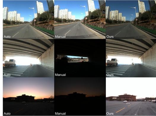
Fig. 1: Images are captured in different illumination conditions. From the left to the right, a camera built-in auto-exposure method, a manually tuned fixed exposure setting, and our method are used. Both the built-in auto-exposure method and the manual setting fail to capture well-exposed images for vision-based algorithms, while our method captures images suitable for the processing of vision algorithms.
