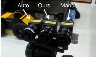
Fig. 4: Camera system for experimental validations. The three cameras had the same hardware specifications and were synchronized using an internal software trigger. Each camera determined exposure parameters using a built-in auto-exposure algorithm, our algorithm, and a manually fixed exposure setting
