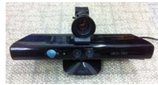
Fig. 2: System setup for real-world shape capture. Flea3 for color images + Kinect for depth images
